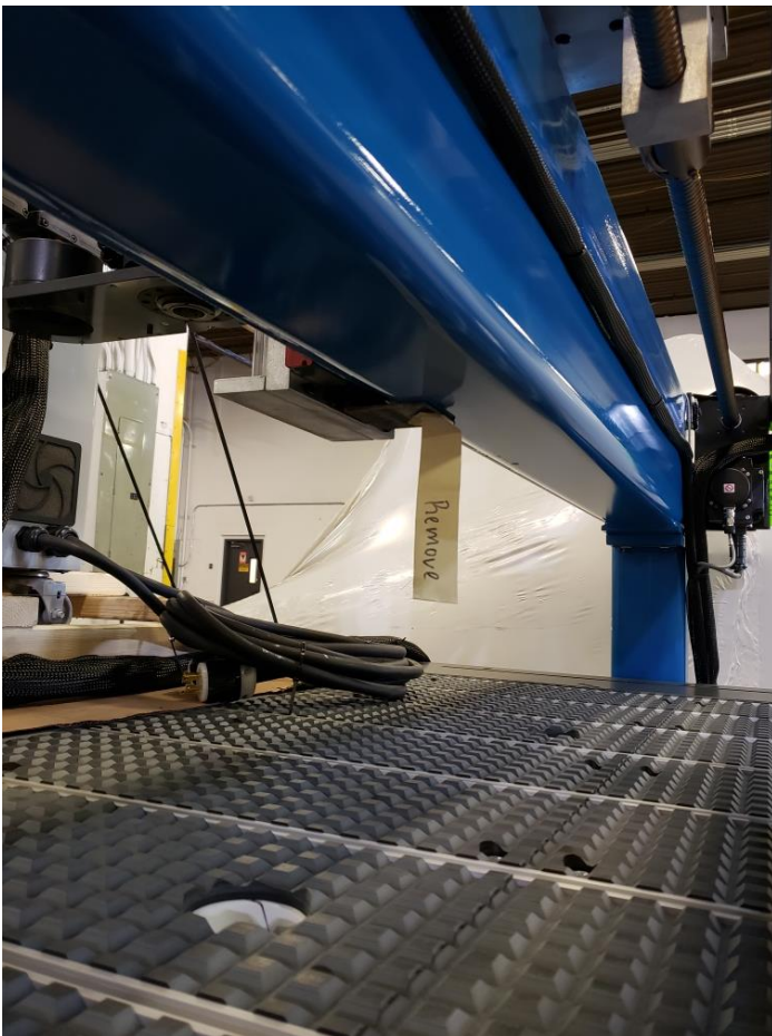
Remove Bolt - Under Gantry
