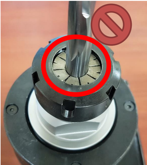
Pictured: The wrong way to install a collet. DO NOT insert a bit before inserting the collet.
