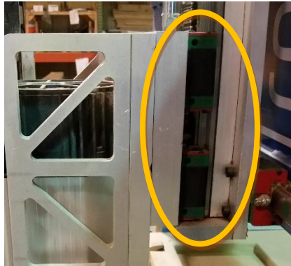
Z axis linear bearings inside the spindle cover on both left and right sides of the Z assembly
