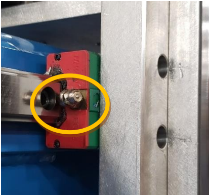
X axis linear bearings on the front of the gantry
