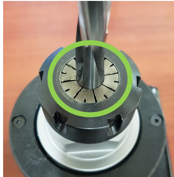
Pictured: The right way to install a collet. Install the collet fully seated into the nut BEFORE installing the bit. Tightening is the last step. The following page shows this step by step.
