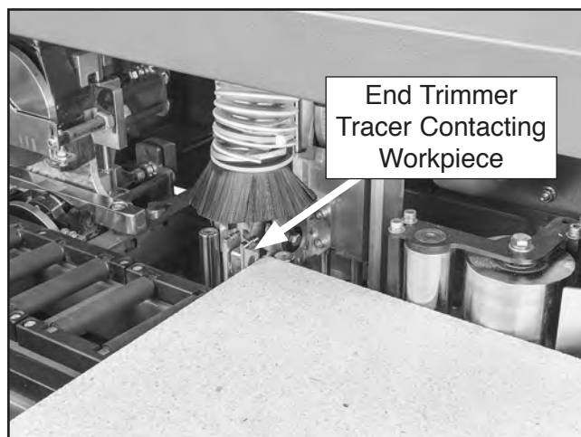
Figure 101. Checking alignment of right end trimmer blade.
