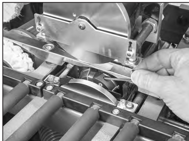
Figure 87. Loosening gib screw to change flush-trimmer knife.
