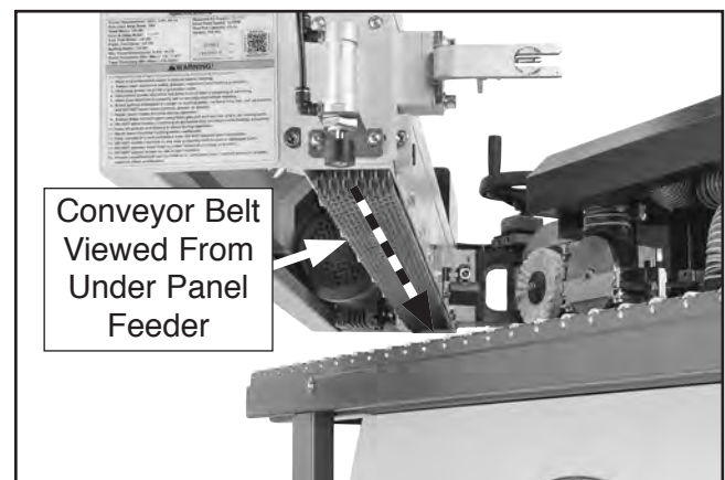
Figure 62. Location of conveyor belt (panel feeder shown in open position for illustration purposes).
